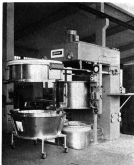
Fig. 2 — Fluid bed granulator WSG 120 opened (Manufacturer's photo: Fa. W. Glatt, 7859 Haltingen, West-Germany).
