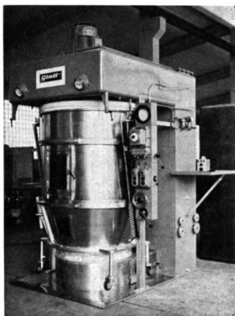
Fig. 1 — Fluid bed granulator WSG 120 closed (Manufacturer's photo: Fa. W. Glatt, 7859 Haltingen, West-Germany).
